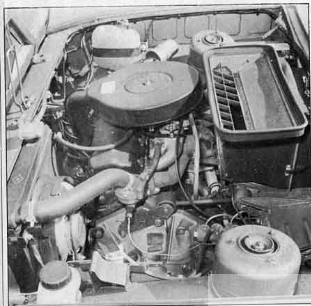
Bonnet opens to reveal sideways-placed Fiat 124 power unit. Note the massive heater air intake box, the MacPherson strut "turrets" and the electric fan
